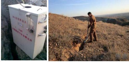
Figure 4: Detection of air leakage pathways using SF<sub>6</sub>.
