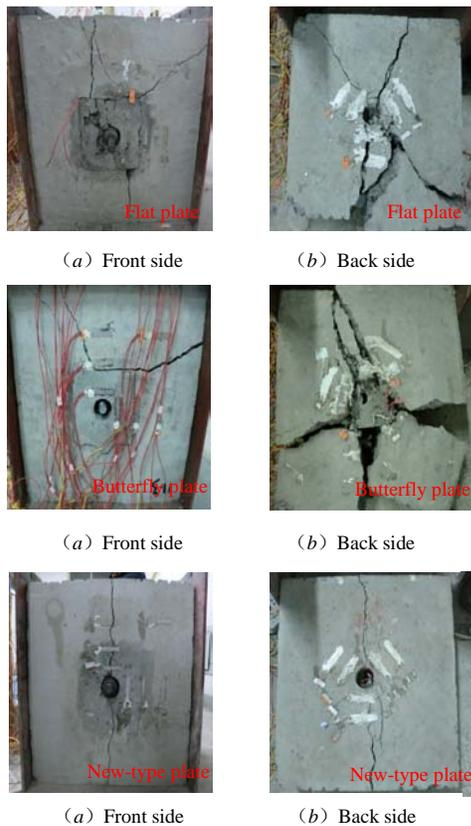
Figure 7. Fracture morphologies of C20 plain shotcrete linings
