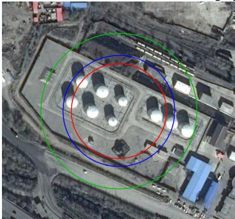
Figure 3: Influence area of pool fire of gasoline tank (each  $1 \times 10^4 m^3$ ).
