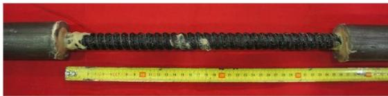
Figure1: Black dowel with ends encapsulated in 450 mm long tubes used for tensile strength testing.
