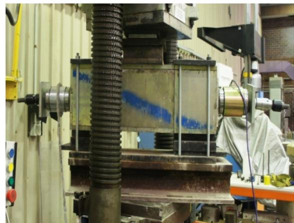
Figure 4: Arrangement of shearing apparatus on compression machine.
