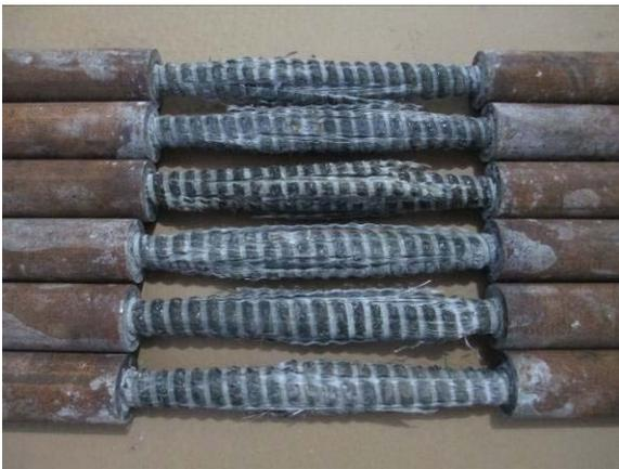
Figure 5: The splitting failure mode.
