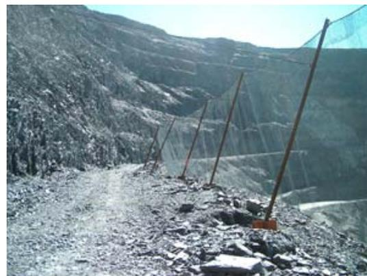
Figure 7: Catch fence installation along bench.
