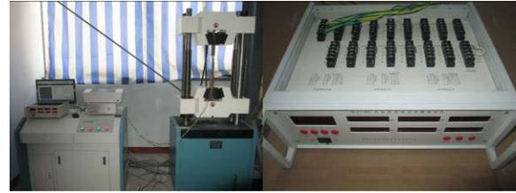
Figure 2: WAW-600B type electro hydraulic servo universal testing machine and XL2118C type stress-strain comprehensive parameter testing instrument.
