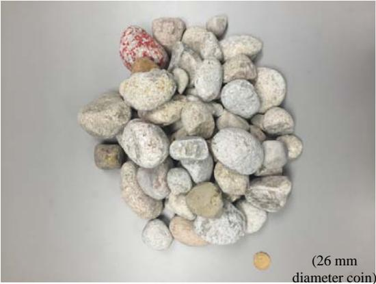
Figure 1: The river pebbles used in the experiments.
