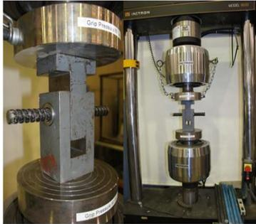
Figure 8: Double shear guillotine apparatus set up.
