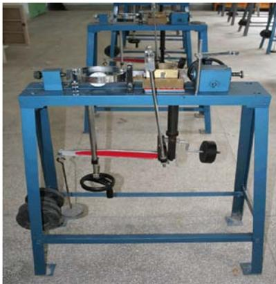
Figure 2: The direct shear apparatus.
