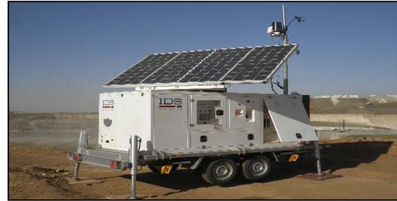
Figure 15: IBIS-FMT slope monitoring radar in action.
