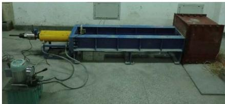
Fig.1. The self-developed multi-function bolt mechanical test system
