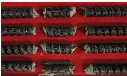
Figure 10: Failure pattern of samples in steel double shared apparatus.
