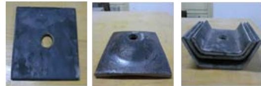
(a) flat plate (b) butterfly plate and (c) new-type plate.
