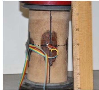
Figure 8: Paste backfill sample equipped with strain gauges.
