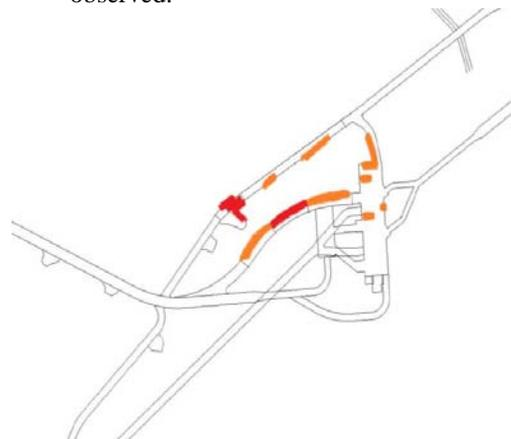
Figure 6: Rockbursts record in the Powerhouse area.
