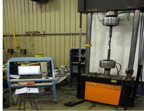
Figure 2: Tensile testing of a dowel in 50 t Instron Universal Testing Machine and monitoring system.
