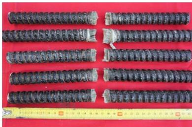
Figure 6: Sheared dowel face with stepped cut.
